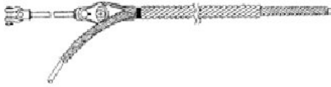
Figure 5-3 Termination for ACCR HTLS Conductor
